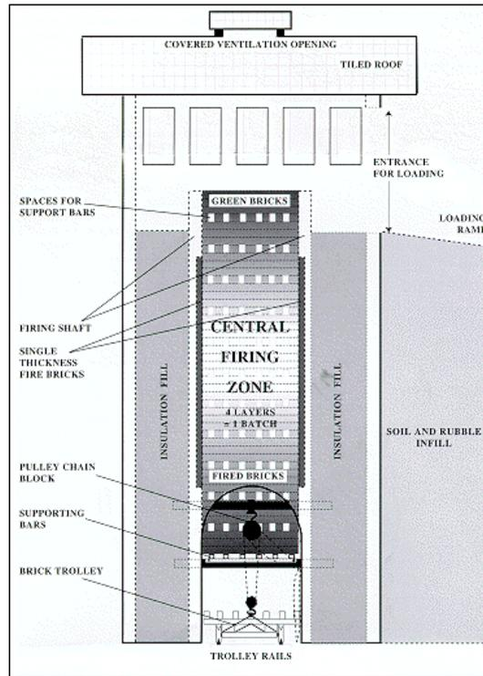
Figure 2 Schematic diagram of a VSBK (reference may be needed if it has been taken from other source)
