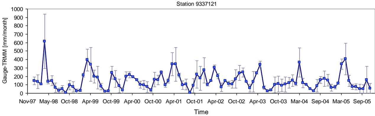
Figure 4 Variation between monthly gauge and TRMM rainfall for the station Osaki forest station
