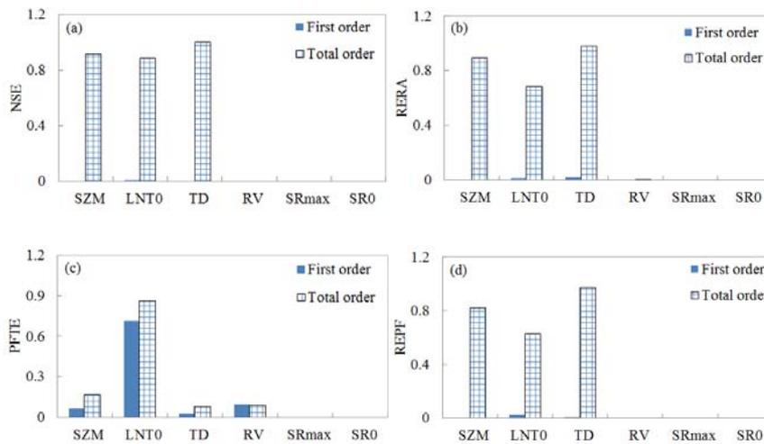
Figure 6 First order and total order sensitivity index of TOPMODEL parameters using the four goodness-of-fit matrices.
